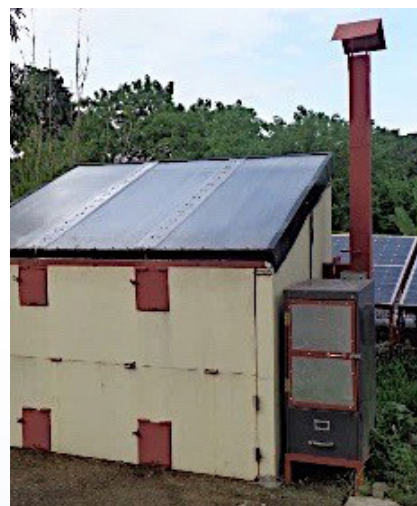
Portable solar powered/heated dryer for wood and non-wood
