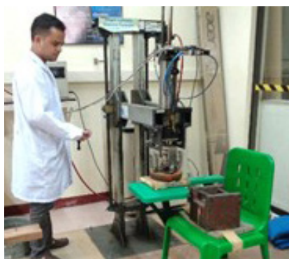
Plastic school tablet armchair for DepEd procurement bidding and upright chair for export undergoing performance and stability testing respectively
