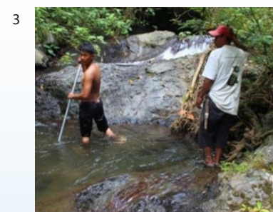
Streamflow and water quality assessment within Aborlan watershed, Aborlan, Palawan (1) width and profile measurement, (2) water quality measurement, and (3) stream velocity determination.
