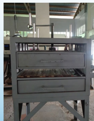
Multi-purpose double acting hot press for engineered bamboo products
