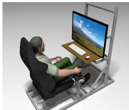
A model of a flight simulator developed by FEATI University which serves as a practice module for pilot training of UAV operators
