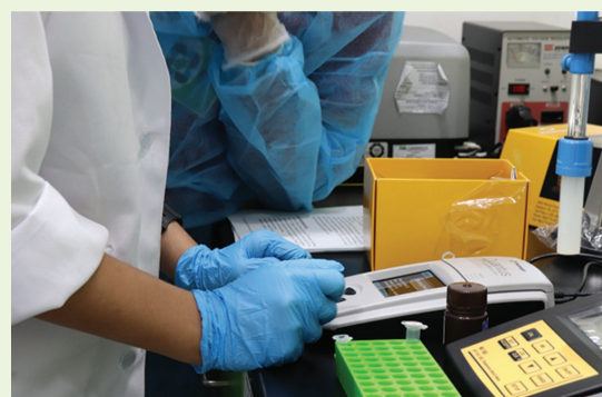
A compact fluorometer is the latest addition in the array of equipment at the NuGen laboratory. The machine can provide a highly sensitive fluorescent detection when determining the concentration of nucleic acids.
