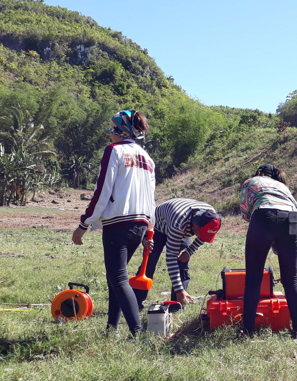
A geo-resistivity survey for groundwater assessment and exploration involves the use of electrical measurements carried out on the ground's surface. A method that determines the depth and thickness of the underlying resistivity layers. Photo courtesy of UP Cebu Center for Environmental Informatics (UP-CENVI).
